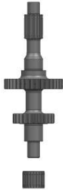
a. Insert the needle roller bearing.
