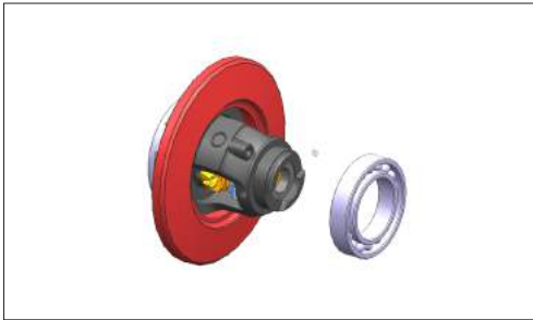
a. Remove the differential cage ball bearing 6011.
