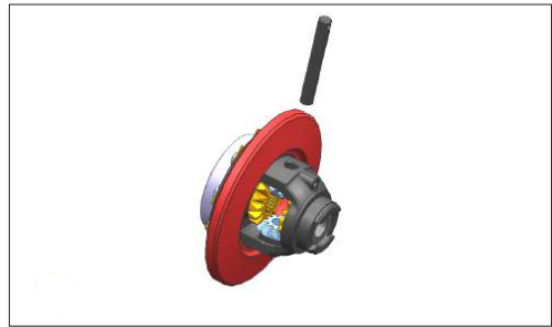
d. Remove the pinion shaft.
