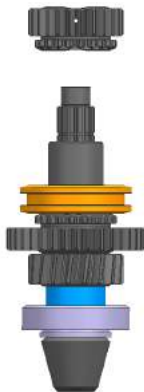
8. Insert the dog gear high.
