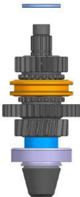
9. Insert the thrust washer.
