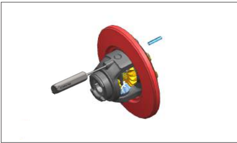
c. Remove the spring cotter sleeve.
