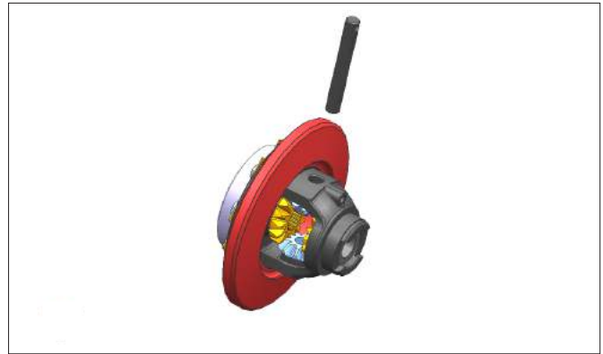
h. Insert the pinion shaft.
