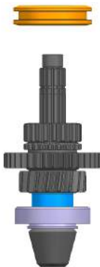
7. Insert the shifter sleeve.
