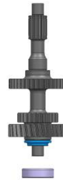
d. Insert the ball bearing 6304.
