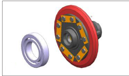
b. Remove the differential cage ball bearing 6211.
